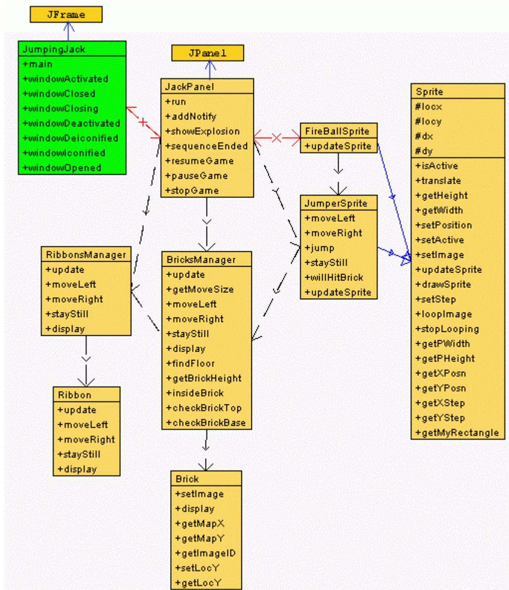
Figure 4. The Core Classes of JumpingJack.
