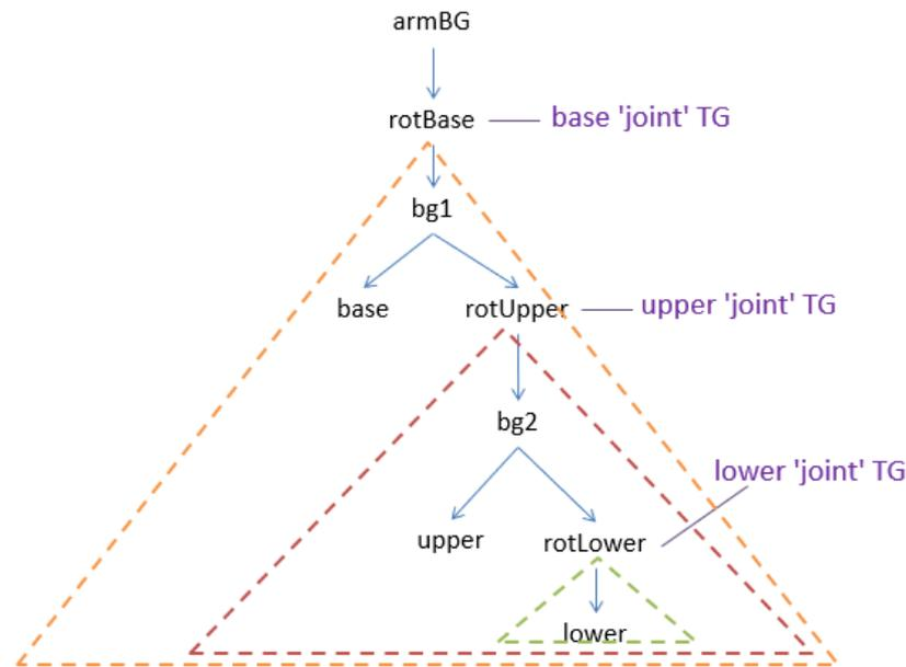
Figure 20. A Partial Scene Graph for the Jointed Arm.
