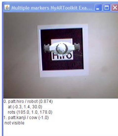
Figure 18. The “Hiro” Marker Upwards, Facing the Camera.
