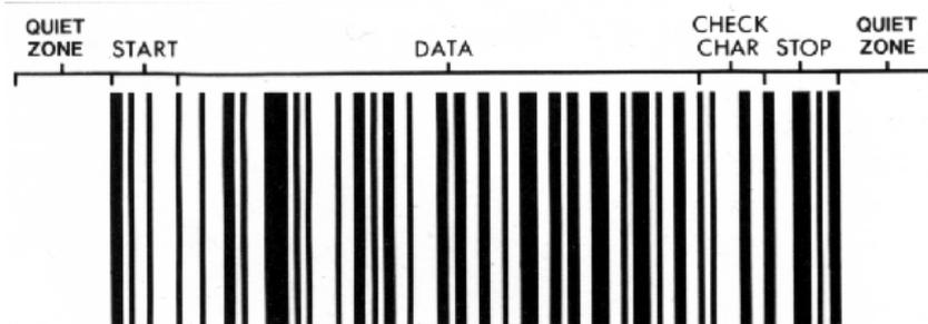
Figure 6. The Elements of a Code 128 Barcode.
