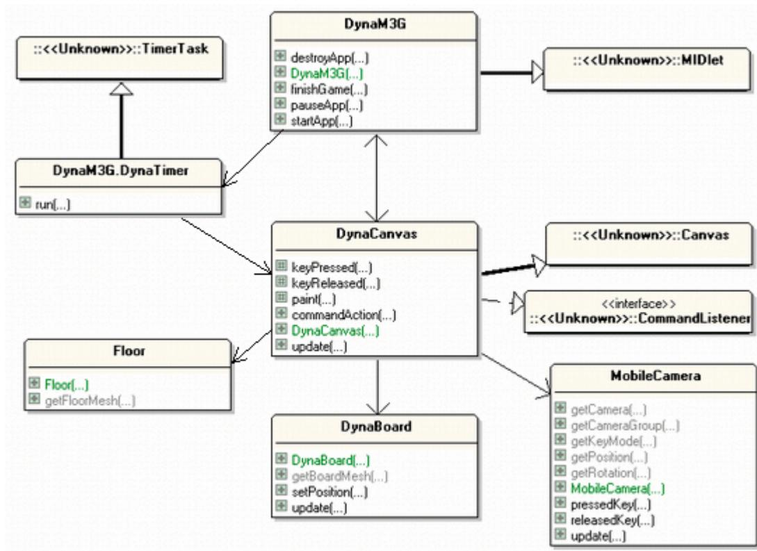
Figure 2. Class Diagrams for DynaM3G.
