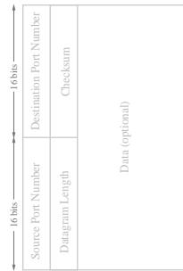
Checksum is the 16-bit one's complement of the one's complement sum of a pseudo header of information from the IP header, the UDP header, and the data, padded with zero octets at the end (if necessary) to make a multiple of two octets.
