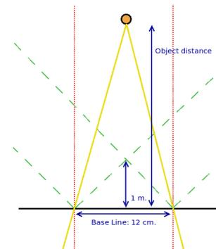
Figure 3. Design of our stereo cameras
