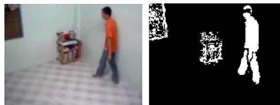
Figure 1: Motion detection and segmentation
