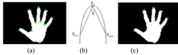
Fig. 4. Fingertip position: (a) key point (b) curvature calculation (c) fingertip points.
