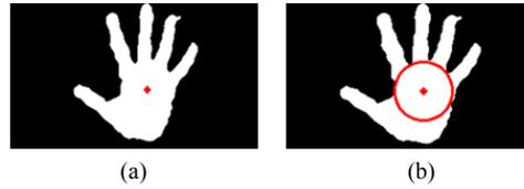
Fig. 3. Initial hand feature: (a) hand center (b) palm size.
